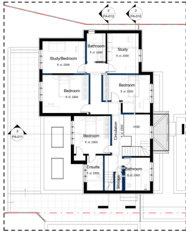
01 - First Floor - As Constructed 1 : 100
